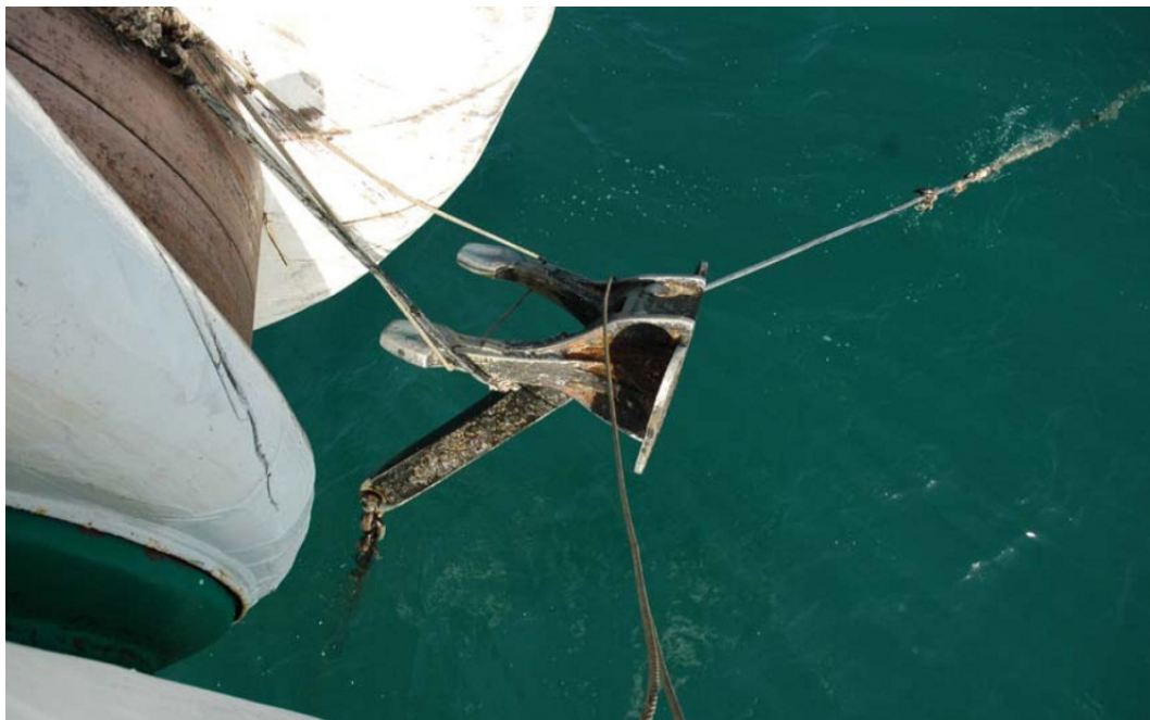
Figure 71: Ships Anchor caught up in cable
