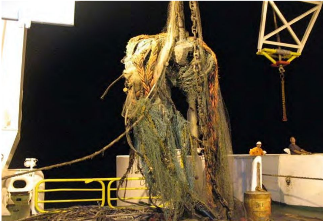
Figure 73: Cable fault caused by fishing gear entanglement
