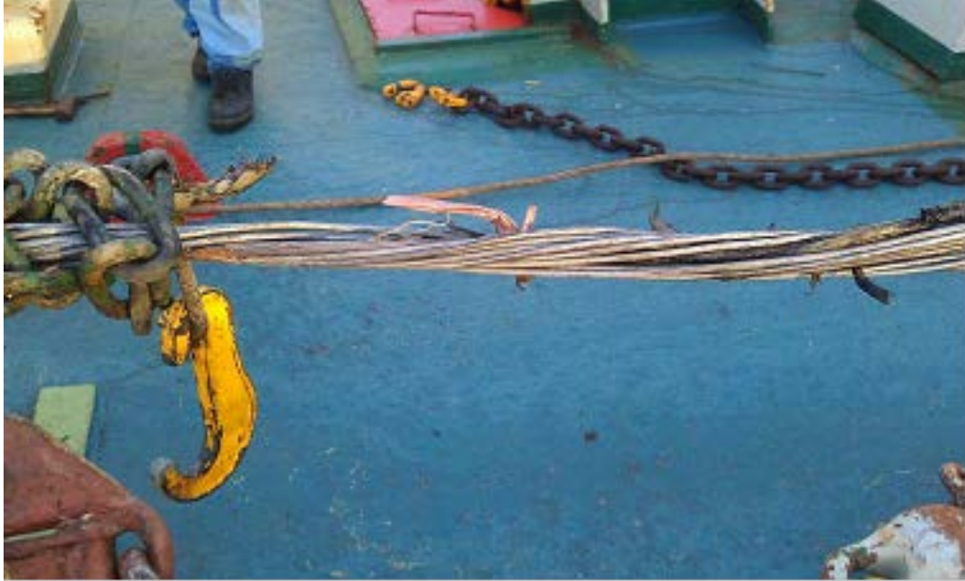
Figure 72: Cable fault with Cargo Lashing chain on cable
