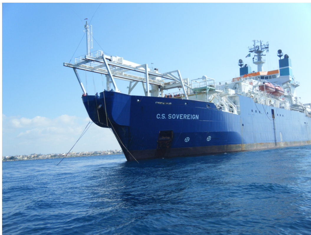
Figure 74: A cableship laying a final bight
