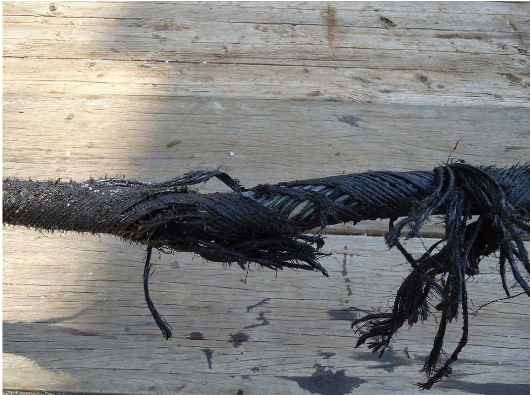
Figure 28: Cable Fault Caused by Fishing Gear (Global Marine)
